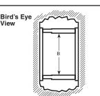
Dimension "B" is "open work area", or the horizontal distance between Struts.
